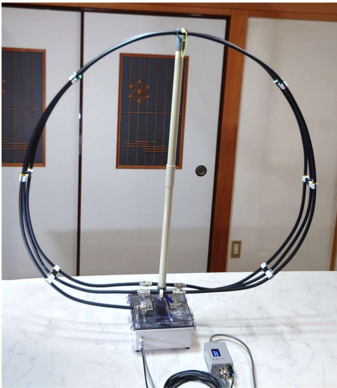
Photo 4 Single Three-turn loop configuration for 80m band
