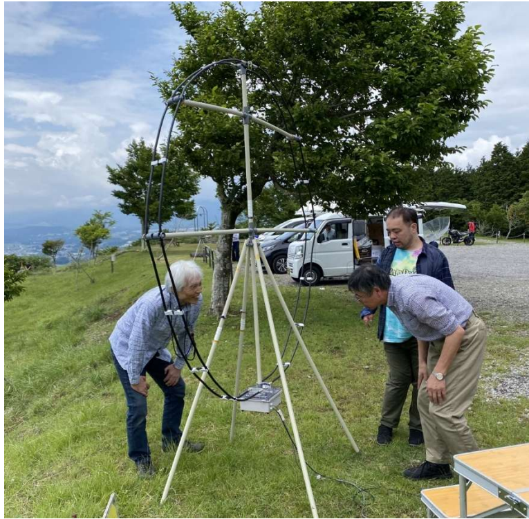
Photo 15 JH1YMC Portable Operation with 2m diameter MLA for 40m band
