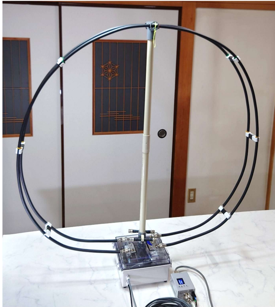
Photo 2 Dual loop, 1m diameter configuration of Desktop MLA
