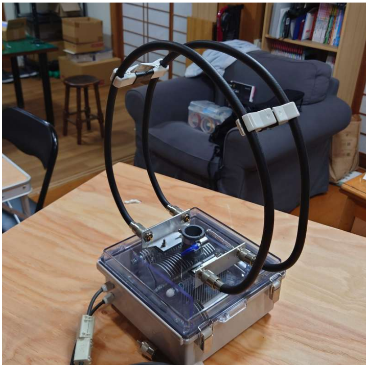
Photo 3 Two loop, 30cm diameter configuration for 6m band
