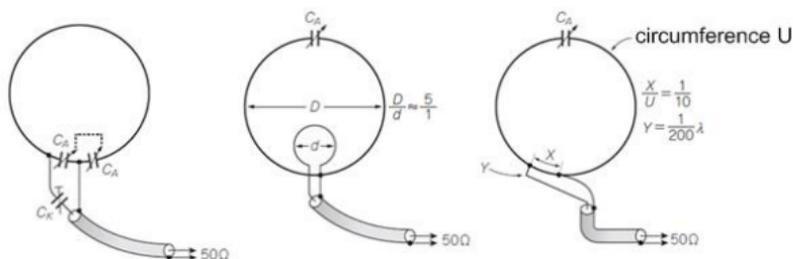
In the early days of MLA, the Patterson method that uses two types of variable capacitors and /or the gamma match methods were used. Currently, the method of electromagnetically coupling a small loop is more popular (the center in the above figure).
