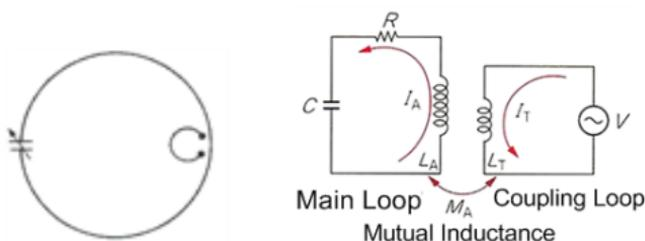
In the equivalent circuit on the right, the ratio of the self-inductance  $L_T$  of the coupling loop and the mutual inductance  $M_A$  between the main loop and the coupling loop is adjusted to  $50\Omega$ . Resolving this circuit for the input impedance  $R_{in}$  at resonance, the equation below is obtained to adjust the Radiation Resistance  $R$  to  $50\Omega$ .  $R_{in} = R \left( \frac{L_T}{M_A} \right)^2$
