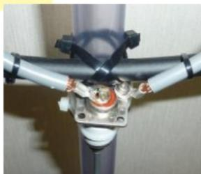
The coupling loop can be a single wire, though it tends to get it a little bigger.
