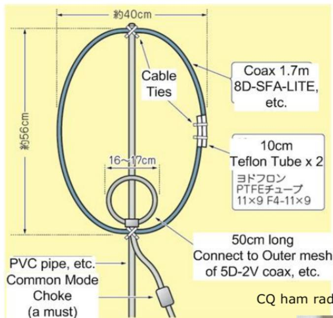
The resonant frequency can be finely adjusted by the position of the clip. It's Okay to be circular instead of elliptical.
