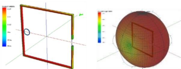
When MLA is installed on the balcony of a steel bar reinforced concrete building, RF current is induced in metals such as handrails and steel frames. When it flows through the entire building, a magnetic field is re-generated and the EM radiation can occur in a complex pattern.
